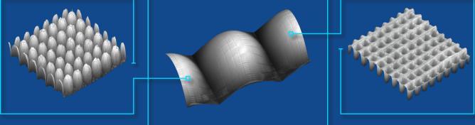
The light-manipulating effects of a combination of micro- and nanoscale plasmonic metamaterials underpin the three optical cues–movement, 3D depth, and multicolor–offered by the KolourOptik<sup>®</sup> Stripe
